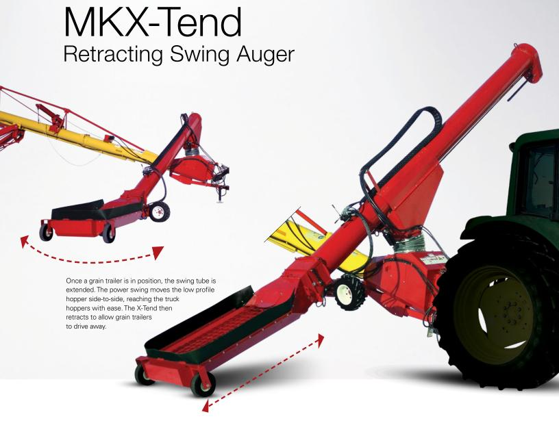
Westfield's retracting swing auger offers the convenience of being able to extend, swing side-to-side and retract, without having to move or reposition the truck. The X-Tend was designed to work with the MKX 130 and MKX 160. It's fast and convenient!
